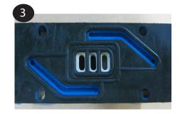
Insert the (4) cap screws (item 1) through the valve body and gasket (items 2 & 10) and place onto the center section (item 8). Ensure the slide valve and valve plate (items 8 & 9) are in place and the valve sits flat on the center section.
