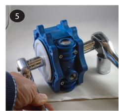
6 Remove the outer plate, diaphragm(s), and inner plate (items 19, 20, 21, 22, & 23) from the side that is loosened. Pull or push the shaft (item 27) and remaining plates and diaphragms out of the center section. If pulling, it may be easier to grip the diaphragm if it is inverted.
