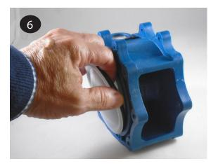
The remaining diaphragm (item 20) and plates (items 19 & 23) may be removed from the shaft (item 27) by hand or by placing the shaft in a vise fitted with soft jaws. Use a 6-sided 5/8" wrench to remove the remaining diaphragm and plates. Soft jaws are required to prevent damage to the shaft. A damaged shaft with result in accelerated o-ring wear. Jaws can be fitted with wood, plastic, rubber, or other soft material to prevent shaft damage.
