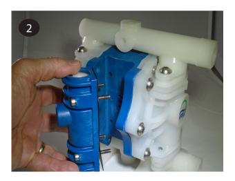
3 Place the new gasket (item 8) on the air valve (item 2) and ensure the slots in the gasket align with the slots in the air valve and valve plate (item 7).
